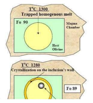
This is what happens to a melt inclusion as it cools. The reverse happens on a heating stage during a microthermometric run. Courtesy Igor Nikogosian.
